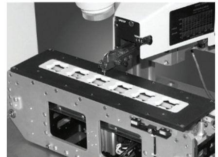
^ ConveyORIZED work stage for fully automated processing.
