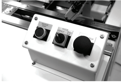
^ Operator panel with inspect and pass through selectable switch.
